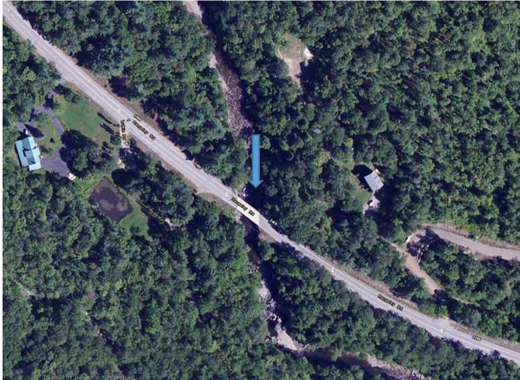
Figure 2. Air photo of bridge crossing showing rapids upstream and bend downstream. Note skew of bridge structure to direction of roadway.
